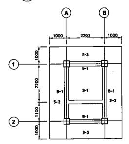
ROOF FRAMING PLAN @ GUARDHOUSE MINAP-BOC-17.004 SCALE
