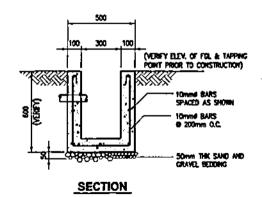
**DETAIL OF RC CANAL** SCALE
